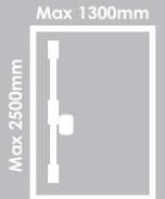
The safety features of this exit device are of fundamental importance to ensure its compliance with standard EN179. No modifications of any kind to the device other than those described in the fitting instructions are permitted.
