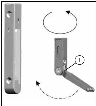
The MULTI Vent must be set to right or left so that Allen screw ① can be accessed to set the braking effect.
