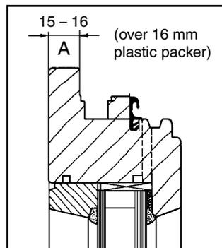
If **dimension A** (rebate height) is greater than 16 mm, the PVC packer supplied ② must be installed below the locking hook.
