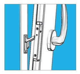
Your windows have been fitted with a Maco Multi Vent Restrictor. The Multi Vent restrictor enables you to control the amount of fresh air entering through the window
