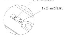
If available always use a drill punch to mark drilling positions using the pencil marks as a guide. The indent made by the point will ensure the drill does not slip.
