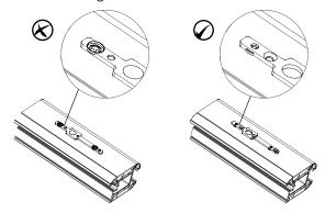
If fitting to PVCu profile pre-drill the fixing holes ensuring the drill bit pierces the steel reinforcement. If fitting to timber drill to a maximum depth of 15mm. You will require both a 2mm drill bit and a 5mm drill bit.
