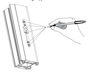
The two holes with washers underneath will require a 5mm drill bit. The three counter-sunk holes will require a 2mm drill bit. 2 x 5mm Drill Bit
